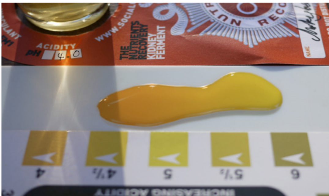
EVERY BATCH OF FERMENTED URINE WILL BE TESTED TO ENSURE ITS ACIDITY IS BELOW pH 4.5
